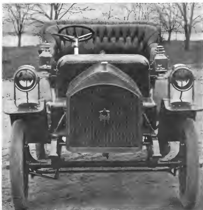
FRONT VIEW OF NORTHERN, SHOWING ARRANGEMENT OF LIGHTS.
